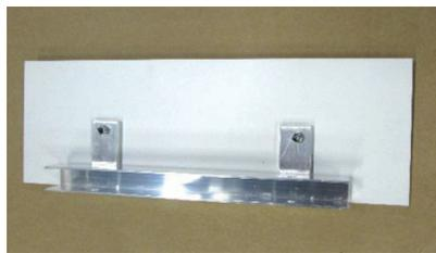
Stick board – projecting to the inside – on the rectangular tube profile and adjust holes. Stick from the outside 2 hexagon socket cylinder screws M6 x 35mm, DIN 912 and screw from the inside 2 self-locking nuts M6, DIN 986. Tighten them (see bottom pictures).
