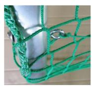
d) Cut the attached cord in half so that there are 2 short cords. Fix the end of one cord in one upper ring nut and knot it well. Pull the cord through the net meshes and fix it in the 2nd upper ring nut and knot it well. Repeat the steps with the 2nd cord in bottom ring nuts.
