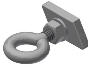
1. Screw on the thread of the eye screw (4) two hexagon nut (5), two washers (6) and two thread plates (7) - initially loose
