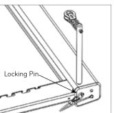
10. Reinsert locking pins until the metal ring touches the frame. You may need to jiggle or slightly lift or rotate the riser to get the locking pins in all the way.
