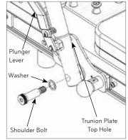
While continuing to support the footbar, release the footbar plunger levers to engage the trunnion plate. Be sure the pins on both sides are engaged. See Figure E.
