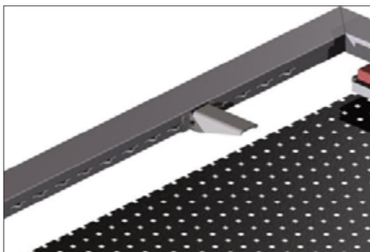
The metal angles shown on the left serve as a stilt for the screwed screen printing boards. The accordingly equipped frame profiles have to be mounted with the closed side of the angle pointing upwards.
